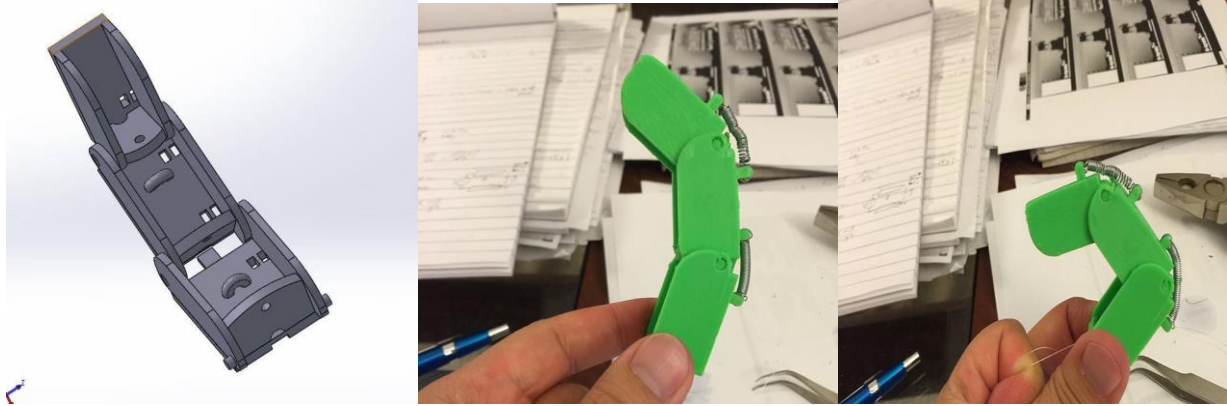
Fig. 6. From left to right: CAD model of a digit including the proximal, intermediate, and distal phalanges; 3D printed digit held in extension by the springs; 3D printed digit in flexion due to tension in the string.
